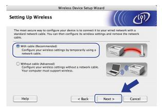
8 Connect the Brother wireless device to your access point using a network cable and click **Next**.
